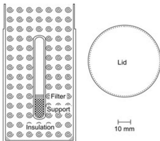
Fig. 1: Experimental setup for HTCAF with insulating “thermos” and quartz ampoule.
